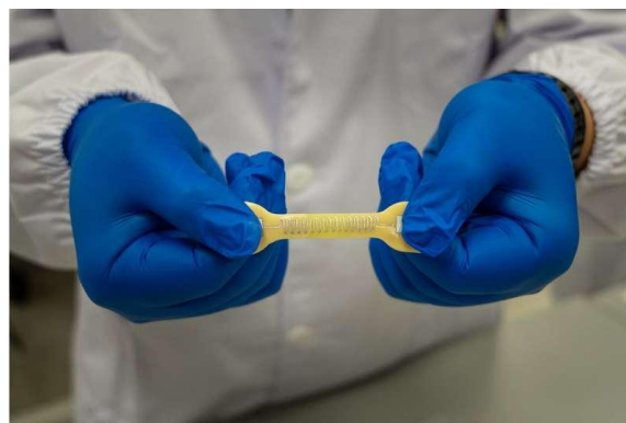
This substrate can withstand a great deal of stretching without breaking apart.
