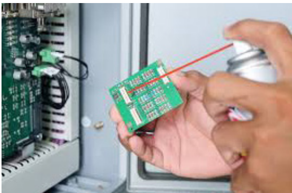
Technicians can use chemical sprays to remove silver tarnish on critical electronic components.
